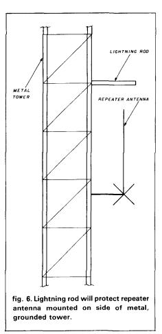
performance, but it will help to protect the antenna and the equipment attached to it during a nearby storm.
