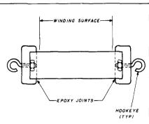
fig. 5. Loading coil can be made up of PVC-type plastic pipe and end caps. Hookeyes permit connection to the antenna wire. tions can be wrapped around the antenna wire and then unwrapped and left to hang down when operation is desired over a lower frequency range.
