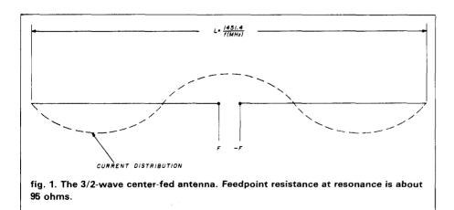
This simple antenna is recommended as a general coverage, single-band antenna for the Amateur bands between 10 and 30 MHz.
