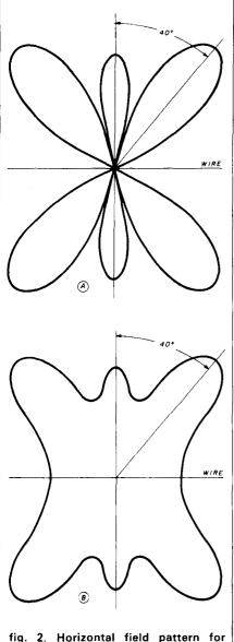
fig. 2. Horizontal field pattern for 3/2-wave antenna: (A) ideal pattern; (B) over imperfect ground.
